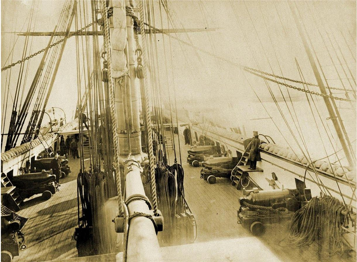
*Figure 16 - Running rigging and shrouds "Hawser-Laid", right-handed. Breeching rope left-handed. Russian frigate, Osliba, ca. 1863*
