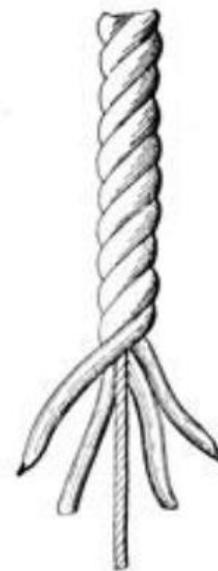
**Back-handed Rope.** In making the plain laid, it was said that the readyes were left-handed, the yarns and the rope itself being right-handed. If, instead of this, the ready is given the same twist the yarn has (right-handed), then, when brought together and laid up, the rope must come left-handed. This is called left-handed or back-handed rope. It is more pliable than the
