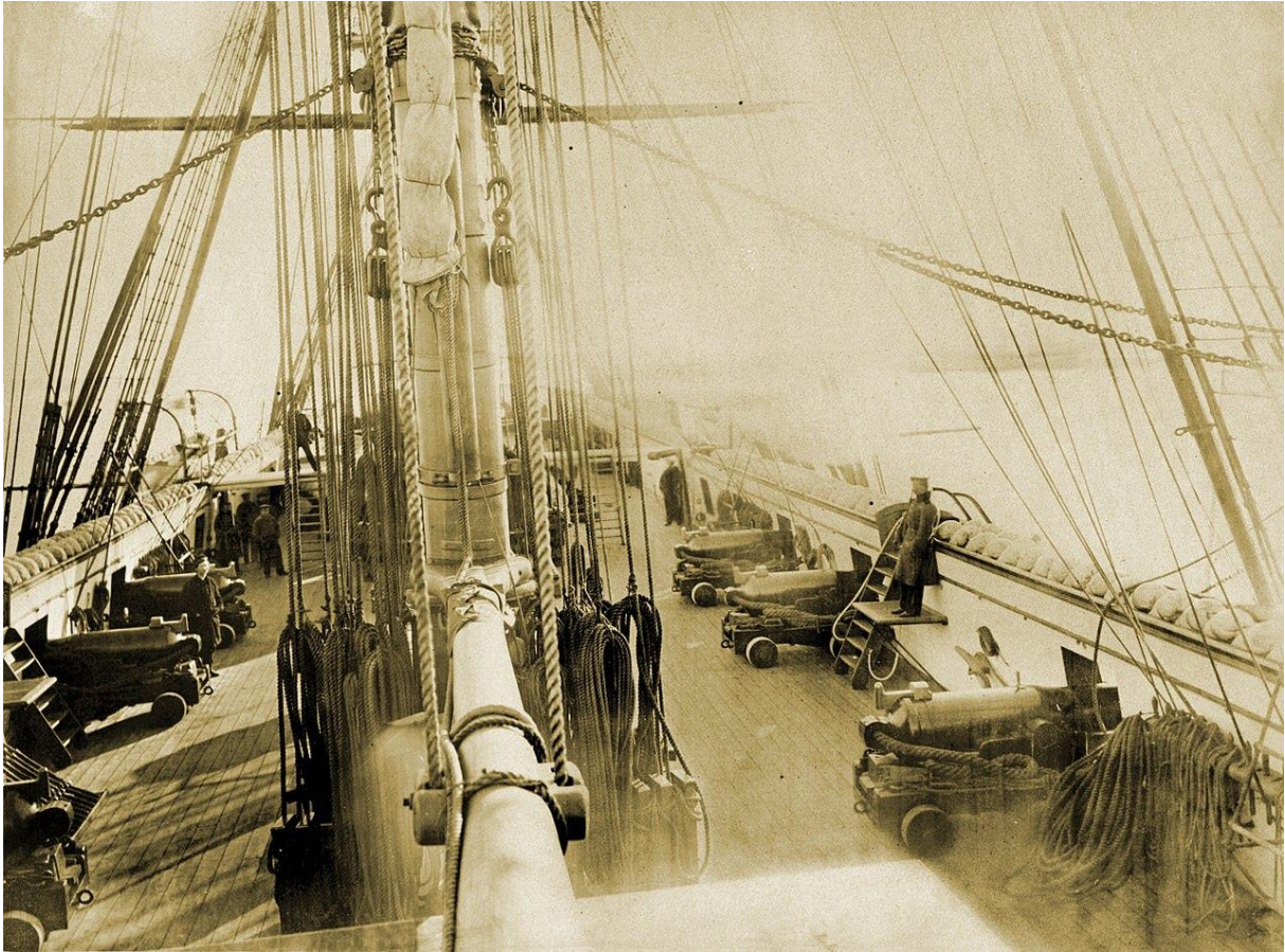
Figure 16 - Running rigging and shrouds "Hawser-Laid", right-handed. Breeching rope left-handed. Russian frigate, Osliaba, ca. 1863
